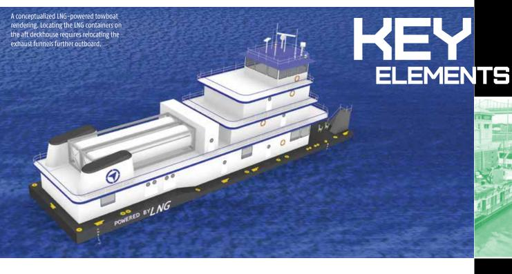
standard approach for LNG conversions is to replace the vessel's engines with a medium speed dual-fuel package. While this approach has a proven track record for retrofitting other vessel types, on certain linehaul towboats this will not be a feasible retrofit.
