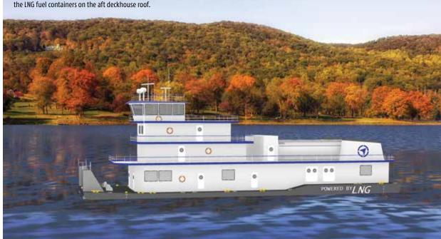
towboat would enable the LNG containers to be shifted further forward, in relation to the vessel's longitudinal center of gravity, to avoid exacerbating the towboat's existing stern trim.
