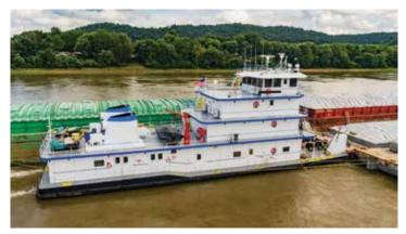
A towboat pushes a barge train down the Mississippi River. Note the loaded hopper barge being towed "on the hip." The Z drives on this barge force the exhaust funnels further aft. An LNG conversion would require relocating these structures.
