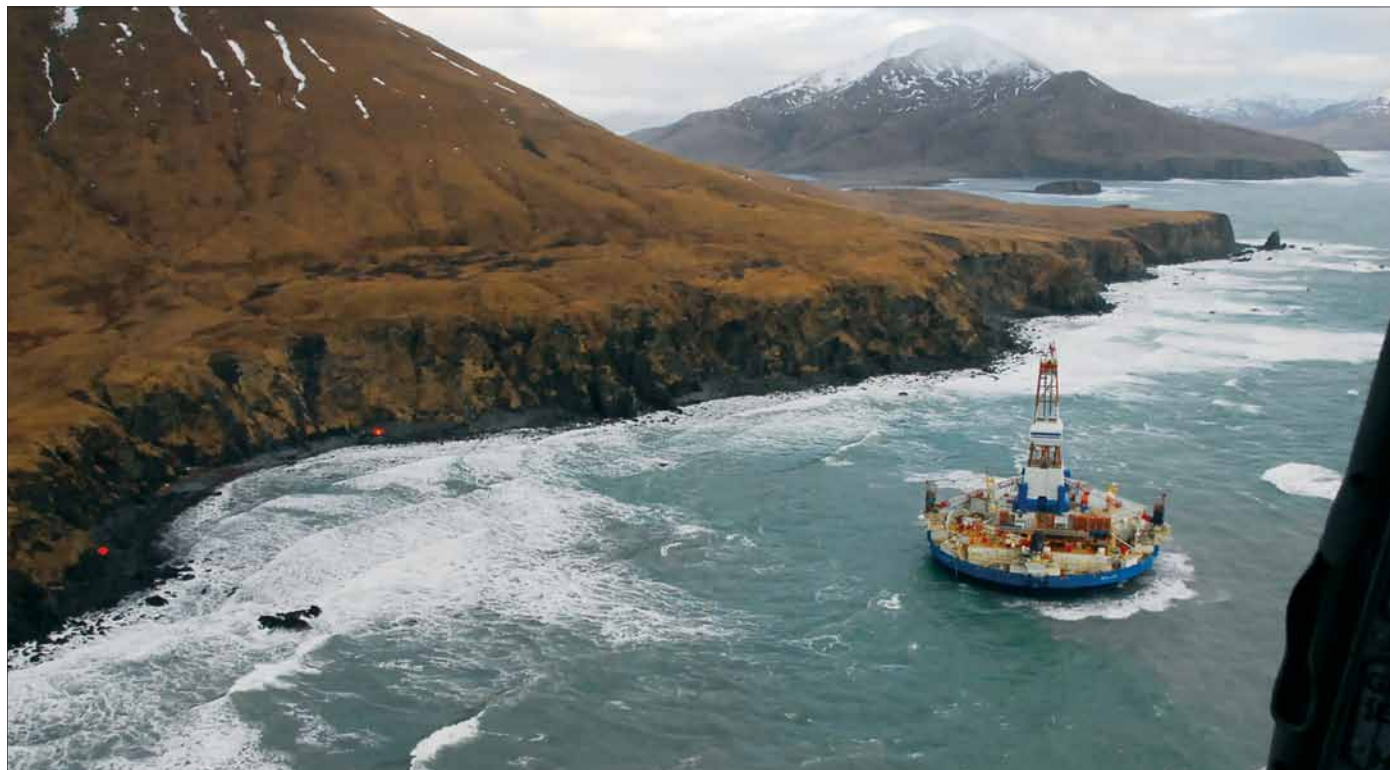
Three life rafts—two pictured—lie on the beach adjacent to the mobile offshore drilling unit Kulluk southwest of Kodiak City, Alaska, on January 3, 2013. The Kulluk grounded after many efforts by commercial towing vessels and a Coast Guard cutter to move the vessel to safe harbor during a winter storm on a tow from Dutch Harbor, Alaska, to Everett, Washington. Coast Guard photo by Petty Officer 2nd Class Zachary Painter
