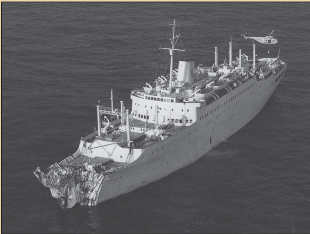
A Coast Guard helicopter helps evacuate patients from the stern of the damaged Swedish liner MS Stockholm after her collision with the Italian passenger liner SS Andrea Doria . The bow of the Stockholm is a broken twisted mass of steel as a result of the collision. Coast Guard photo
