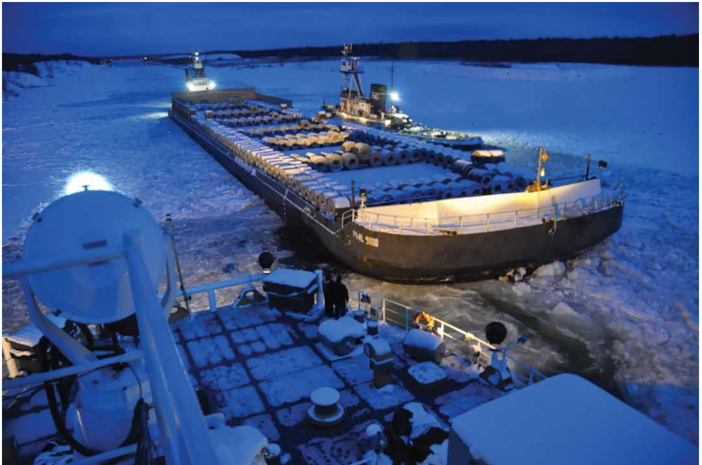
The crew of the Coast Guard Cutter Mackinaw approach the barge PML 9000 backward to use the cutter's prop wash to help break the ice around the barge after it became stuck in the St. Marys River in December 2013. The Mackinaw's crew freed the barge and both of its escort tugs. Coast Guard photo by Ensign Michael Cooper
