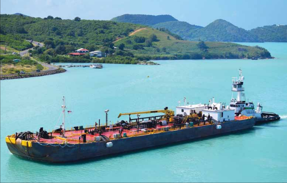
The M/V Brandywine and barge Double Skin 141 , an articulated tug-barge unit. Photo courtesy of The Vane Brothers Company
