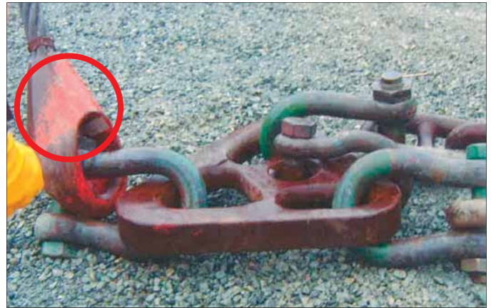
Arrangement of critical towing components in the yard in Dutch Harbor, Alaska, just prior to the departure on the accident voyage. The red circle indicates the critical component that failed, leading to the loss of the tow on the morning of December 27, 2012. Coast Guard photo
