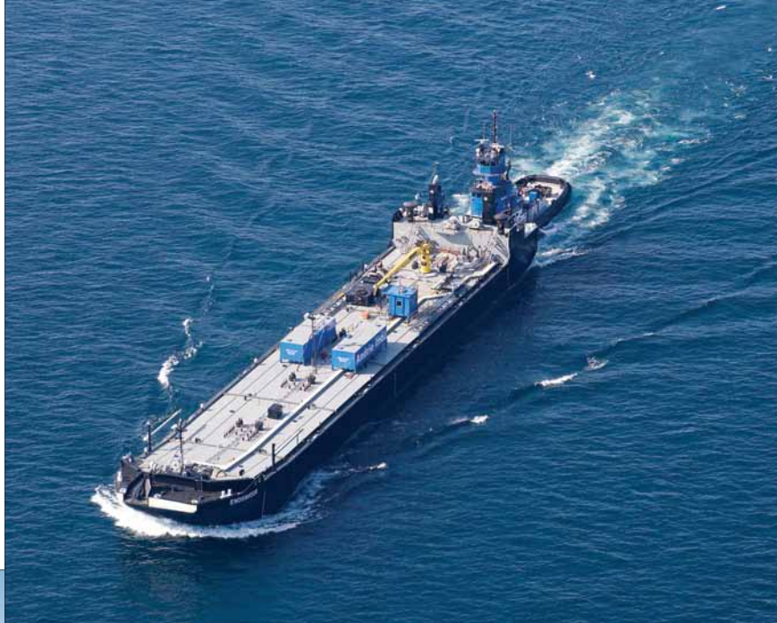
The M/V Karen Andrie and barge Endeavour , an articulated tug-barge unit. Photo courtesy of Andrie Inc.
